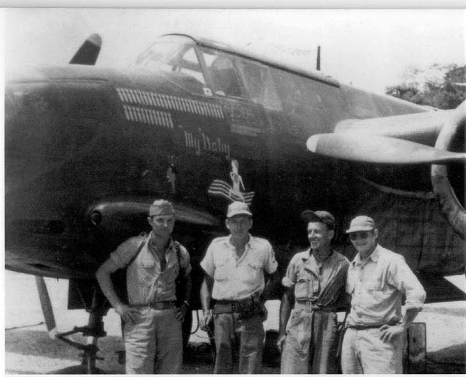
My Baby had completed 39 missions by late 1942 or early 1943. The cooling vents on the cowl indicate that this was an early A-20A. It appears that the glass nose has been painted over indicating that the ship has been converted to a gunship with four .50 caliber machine guns being mounted in the nose. There were only enough A-20s to equip one squadron of the 3rd BG, a situation which did not change until early 1944. (Air Force Museum)
