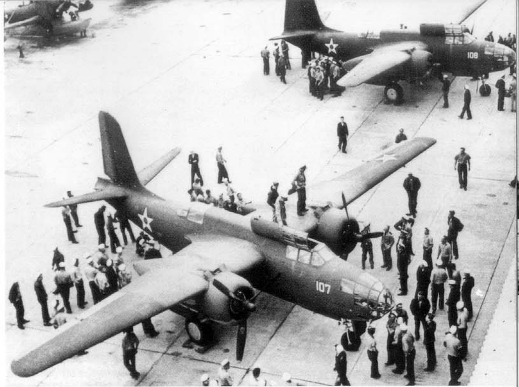
A group of Navy and Marine Corps personnel examine a DB-2, the Navy version of the A-20B, which was used as a high speed target towing aircraft. Eight of these were received by the Navy and operated by the Marines. (NASM)
