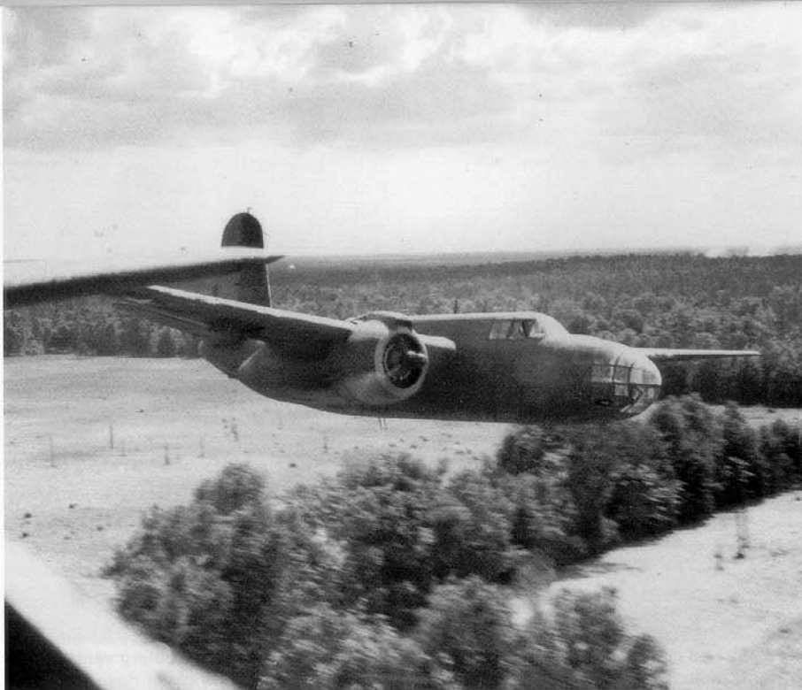
An A-20B Havoc flies low over the Florida countryside during a training flight from the Army Air Force facility at Orlando, Florida. A large number of A-20Bs were used for training due to deficiencies in the design, such as a lack of self-sealing fuel tanks. (USAF)
