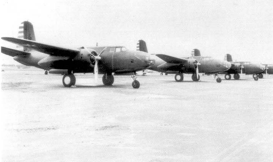
The A-20A went into service in the Spring of 1941 with the 3rd Bomb Group (3rd BG). These early aircraft have the cooling vents on their cowlings and Natural Metal propeller blades (which later were painted Black). None of these aircraft have machine guns fitted in the nose. (USAF)
