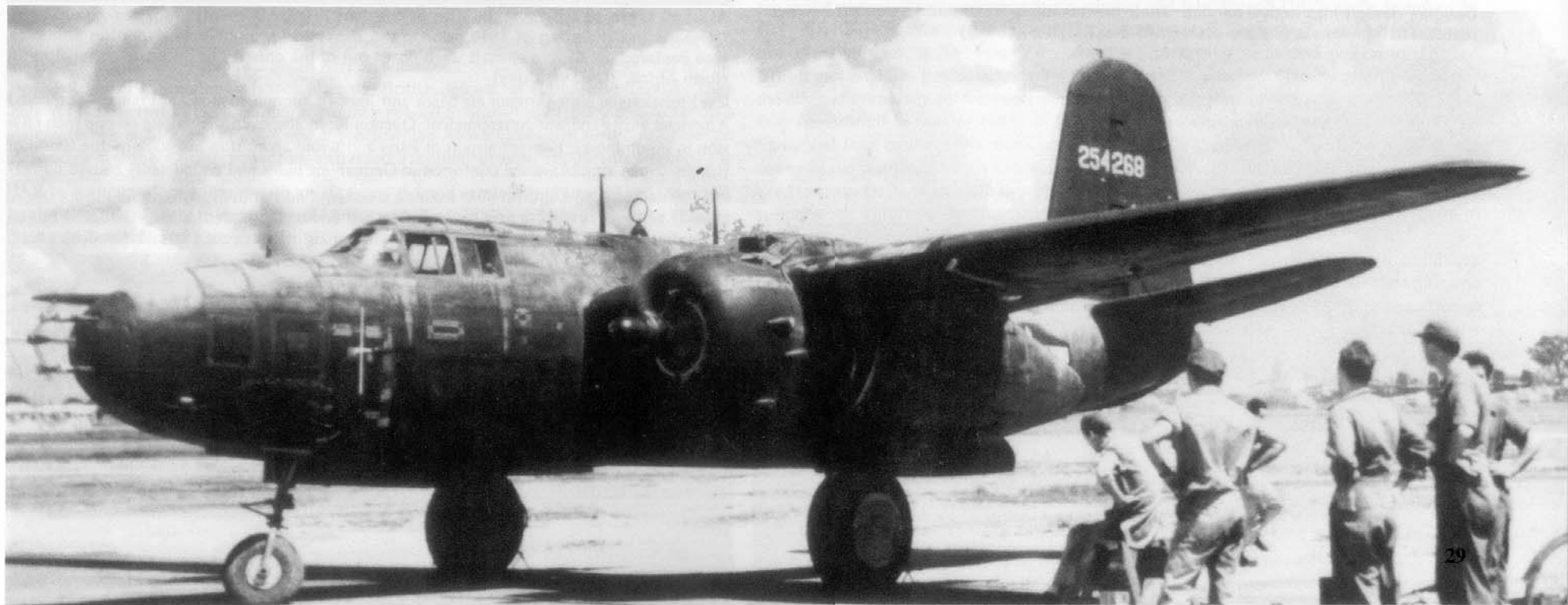
The first P-70 prepares to take off on a night test flight. There are two antennas on top of the wing and an arrow shaped antenna on the nose. The aircraft does not have the ventral cannon tray fitted under the bomb bay area. The first P-70s were converted from the A-20 which had originally been slated to operate with a turbosupercharger. (Air Force Museum)
